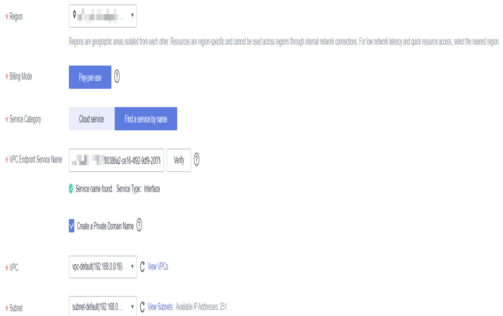
Figure 2-18 Creating a VPC endpoint for SWR
